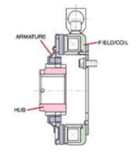
Components used in Electromagnetic Braking system
